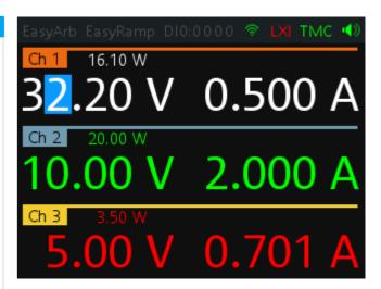
The different operating conditions are marked by colors: constant voltage operation is indicated in green, constant current operation in red, inactive channels are shown in white, a number marked by a blue background indicates that the channel is in setting mode.
