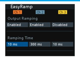
EasyRamp simulates operating conditions with controlled rise of supply voltage to prevent a sudden voltage surge.
