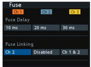
Users can set the power supply so that all channels are switched off if one channel hits the limit. Or it can be set to leave one channel working.
